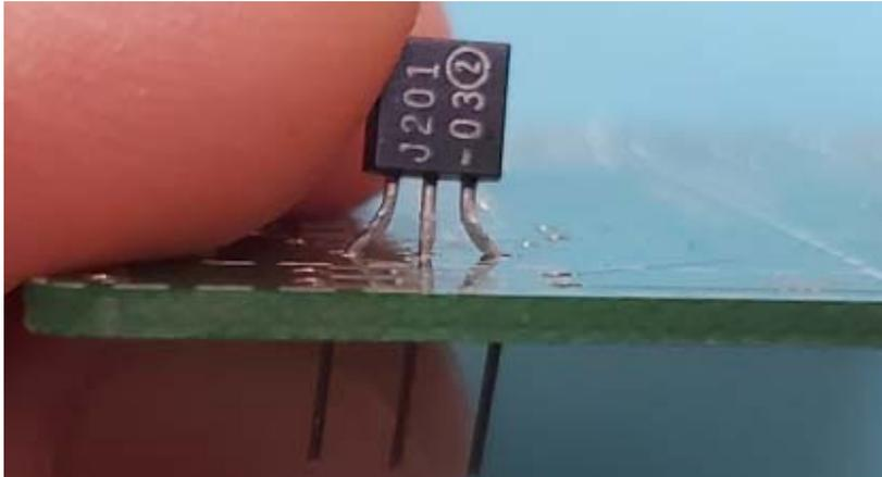
These devices typically only install one way, but pinouts can differ from different part numbers, so if using a different part number transistor than the one called out in the bill of materials will require that you check the datasheet of the transistor and check which legs are what pins for it to function properly.
