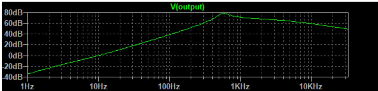
With the Volume pot changed to 100K and the output capacitor changed to 10nF
