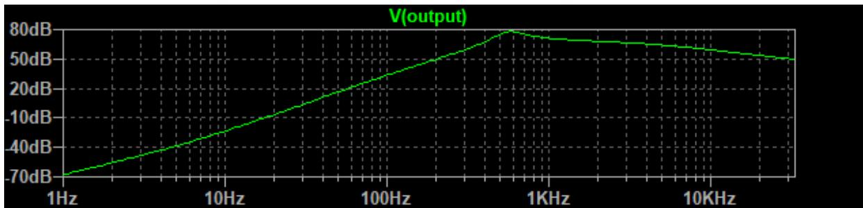
Stock build but with the input capacitor raised to 470nF
